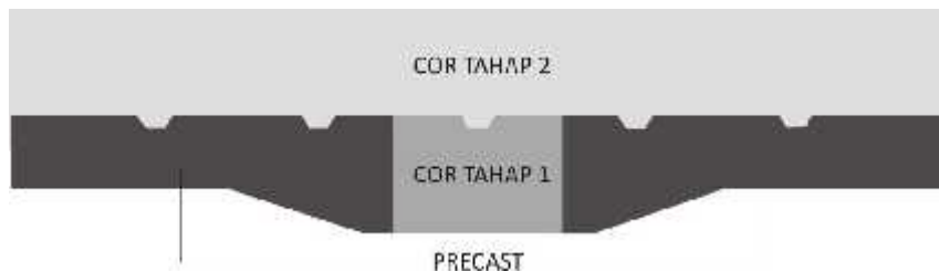
Gambar 14. Ilustrasi Pengecoran Cast in situ Pier head Precast (PT. Waskita Karya,2016)
