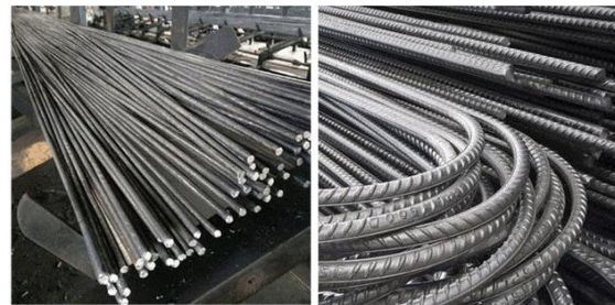
Besi Beton Polos ( Plain Bar ) Besi Beton Ulir ( Deformed Bar )
